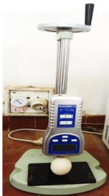
e) Bench top materials testing setup. Figure 1. Duck eggshells and breaking test
