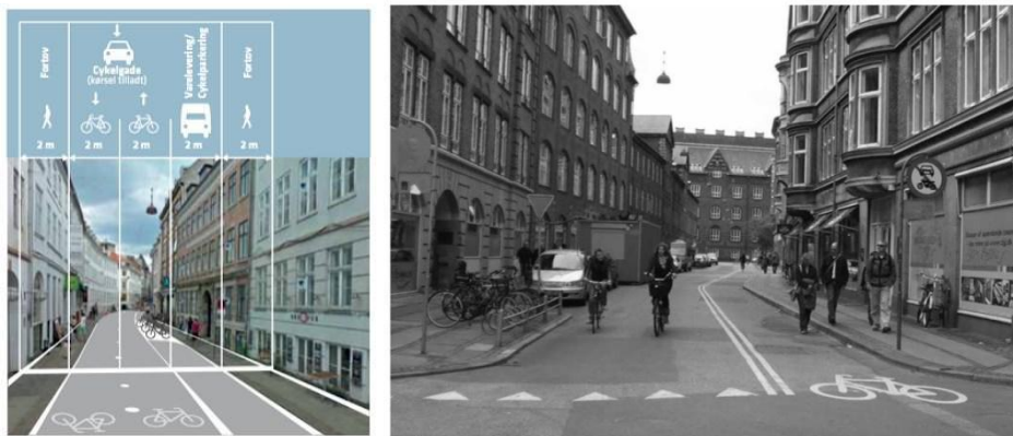
Figure 13. The micro-scale of street design gives the priority to cyclists and pedestrians, in the right; the cycling lane that enables cycling to ride in two directions, while cars were restricted to one direction [31].
