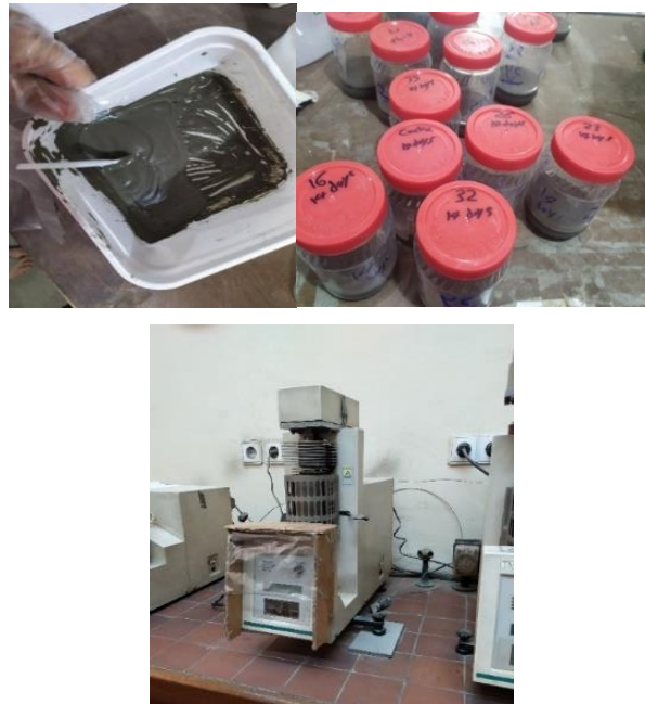
Fig. 10 Preparation cement pastes specimens for TGA test.
