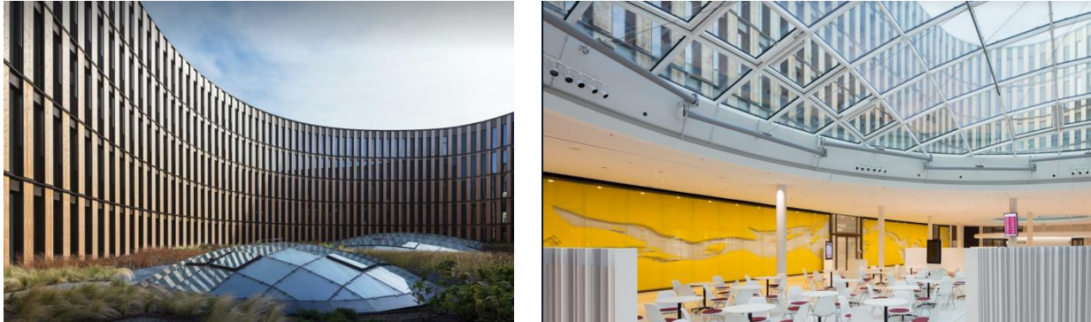
Figure 19: use of skylight and green roof in the internal court. Source: https://archello.com/story/50247/attachments/photos-videos/18
