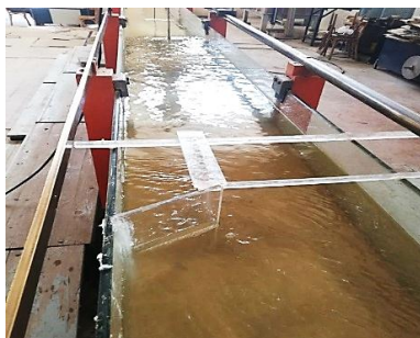
Fig. 4 Setup of Groins model with different orientation angles.
