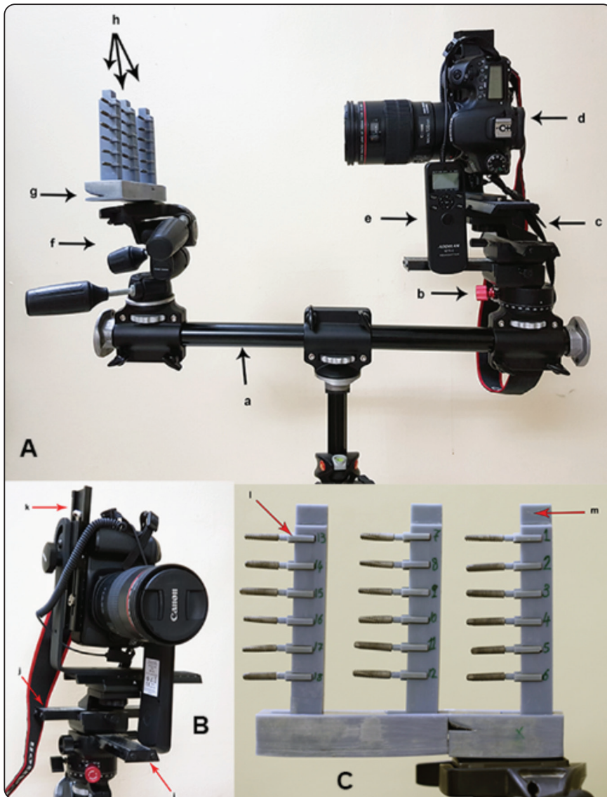
Fig. (1) Section A: a. Horizontal tripod arm, b. 360° rotating tray c. Four-way horizontal macro slider, d. DSLR Camera, e. Remote shutter release, f. Tripod head, g. Implant-photographing tray, h. the three implant-holder trays with 18 implant holders carrying 18 expired implants; Section B: i. Z-axis anterior/posterior slider, j. X-axis right/left slider, k. Y-axis vertical slider; section C: l. implant holder, m, implant-holder tray.
