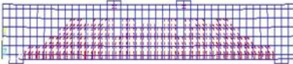
Fig 26. Crack pattern for s50
