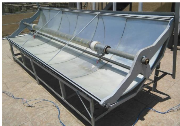
Fig 3 Photographic view of the parabolic trough along with the receiving tube
