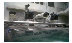
Fig. (2) Sensors mounted on the vehicle
