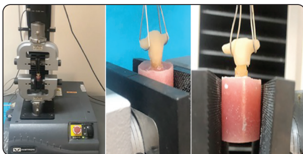
Fig. (2) Specimens in universal testing machine for pull-off test
