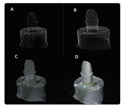
Fig. (5) Reconstruction of three-dimensional model. A: Sparse point cloud, B: Dense point cloud, C: Mesh construction & D: Textured mesh.
