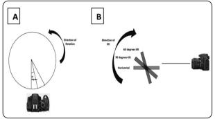
Fig. (3) A: Rotation Step Angle by 10 degrees, B: Tilting angle Horizontal, 30 & 60 degrees.
