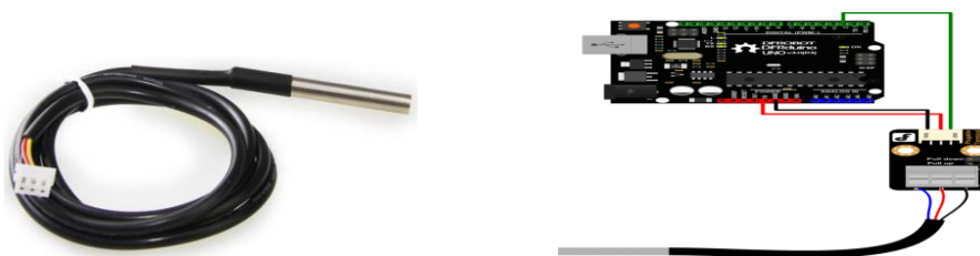
Figure 5: Temperature sensor integration with Arduino
