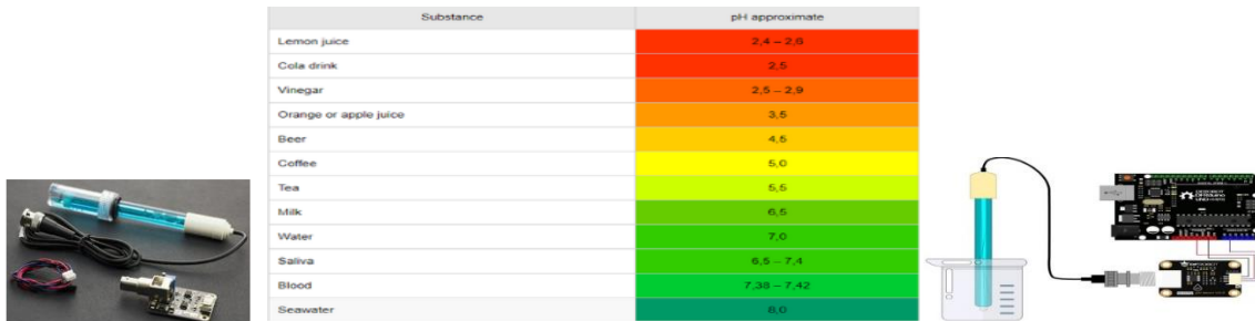
Figure 4: Ph sensor integration with Arduino
