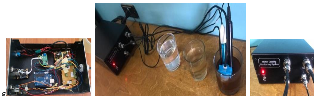
Figure 8: Integration all components with casing and testing
