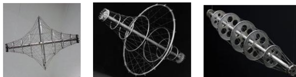
Fig. 14. Stiff Hollow Rope Structure System
