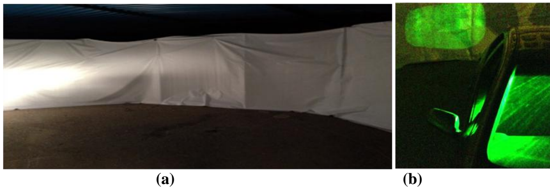
Figure 6. practical FOV testing (a) cylindrical screen. (b) laser backlighting.
