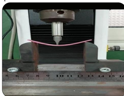
Fig. (4) Flexural strength Test Setup
