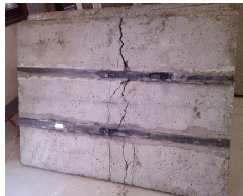
Fig.10 Crack Pattern and Mode of Failure for Slab SSC.
