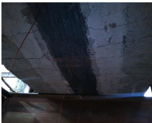
Fig.11 Crack Pattern and Mode of Failure for Slab SSW60.
