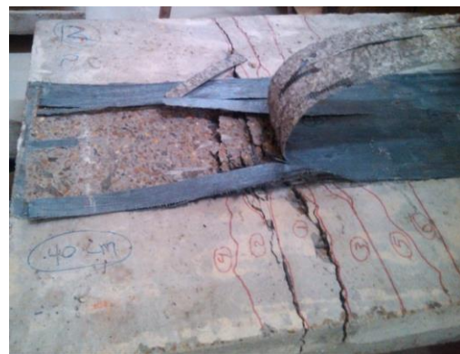
Fig.11 Crack Pattern and Mode of Failure for Slab SSW60.
