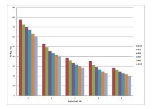
Fig. 5. Effect of engine load and percentage of catalytically cracked used cooking oil in its blend with diesel fuel on the air-fuel ratio.
