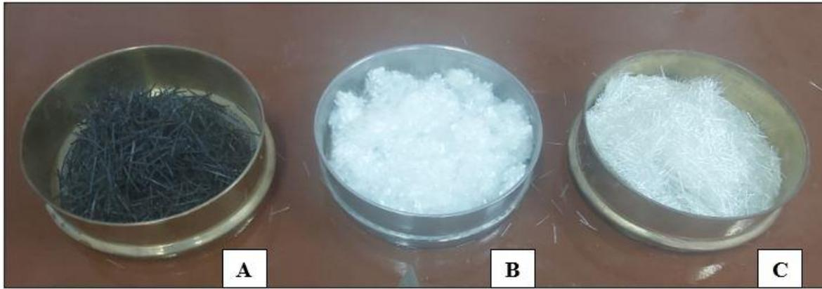
Fig. 1: Three Groups of Fibers, where A) Polyolefin, B) Polypropylene and C) Glass Chopped fibers.
