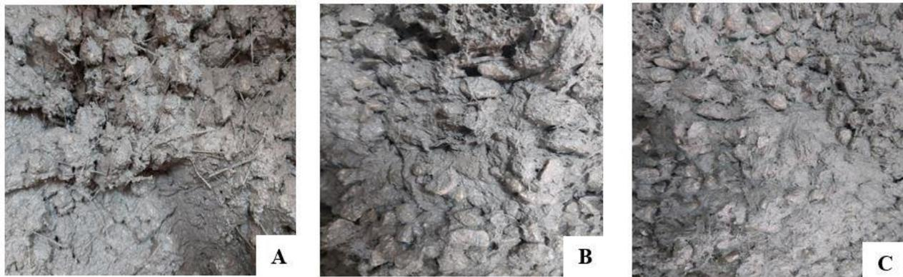
**Fig. 7: Shows the Concrete Mix of the Different Types of Fibers (6 kg/m<sup>3</sup>), where A) Polyolefin, B) Polypropylene and C) Glass Chopped**
