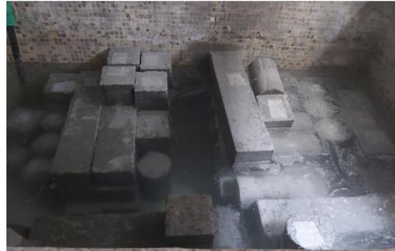
**Fig. 10: All Samples of Different Concrete Mixes After Being Placed in the Curing Basin**
