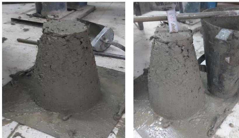
**Fig. 8: Effect of Fiber Usage on Slump Value of Concrete**
