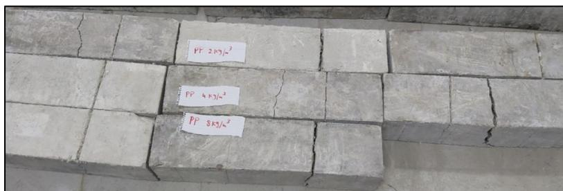
**Fig. 25: The Crack Pattern and Mode of Failure for Prisms with Polypropylene**
