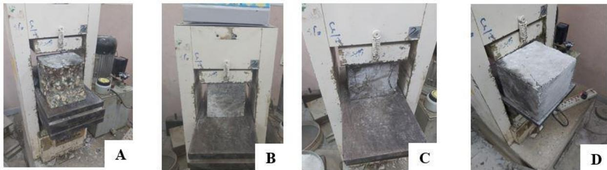
Fig. 14: Compressive Strength Test for Standard Cubes, where A) Fiber Free, B) Polyolefin, C) Polypropylene and D) Glass Chopped.
