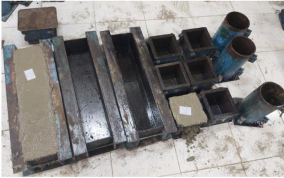
**Fig. 9: Preparing and Concrete Casting Process for each Concrete Mix**
