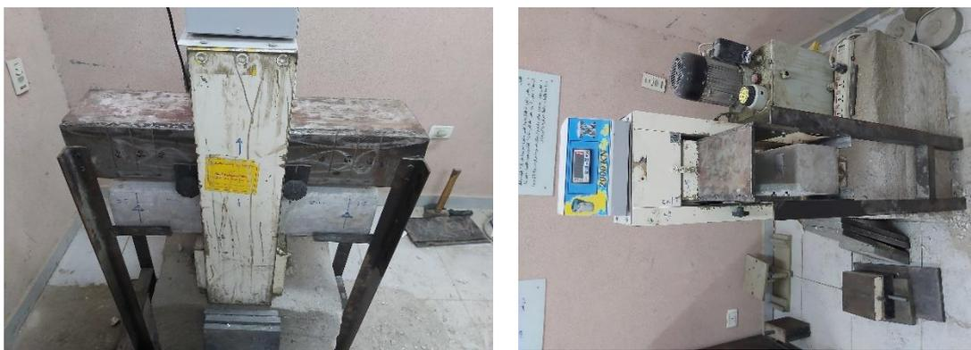
Fig. 22: Flexural Strength Test Setup for Standard Prisms(15cmx15cmx60cm)
