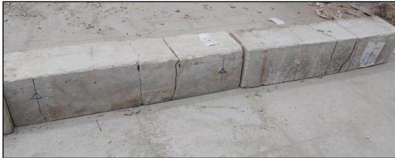
**Fig. 23: The Crack Pattern and Mode of Failure for Control Prisms**
