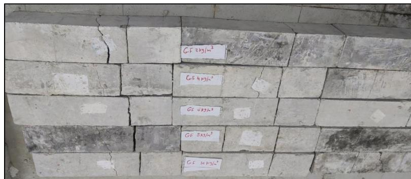
**Fig. 26: The Crack Pattern and Mode of Failure for Prisms with Glass Fibers**
