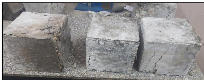
Fig. 15: Non-explosive Failure for Cubes at which  $6 \text{ kg/m}^3$  Polyolefin Dose Were Used
