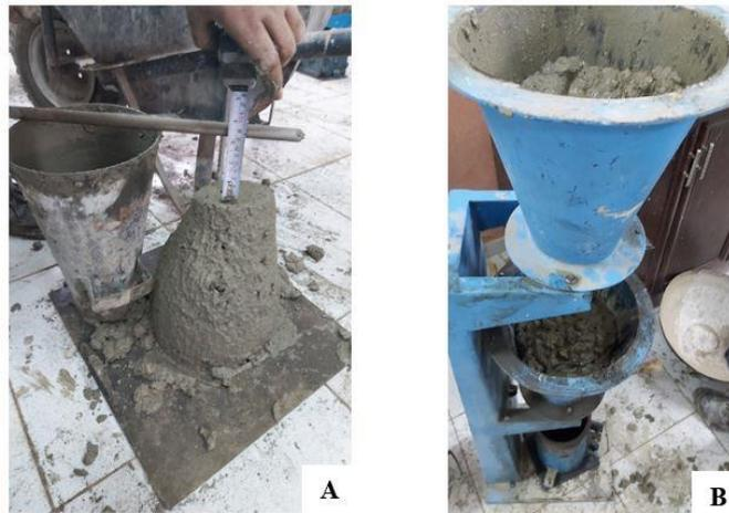
Fig. 4: Presented Slump and Compacting Factor Tests for Control Specimen, where A) Slump and B) Compacting factor
