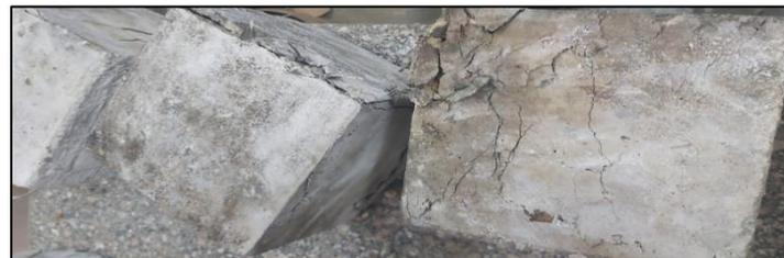
Fig. 17: Non-explosive Failure for Cubes at which 6kg/m<sup>3</sup> Glass Fibers Dose Were Used
