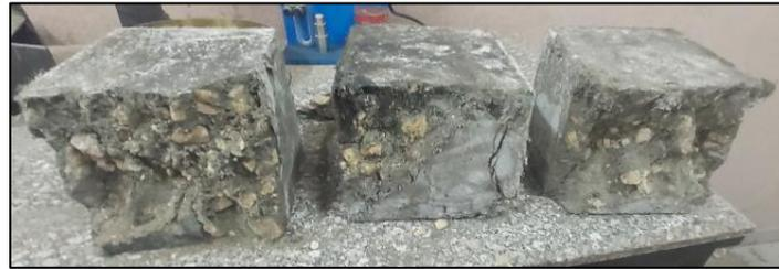
Fig. 16: Semi-explosive Failure for Cubes at which 6kg/m<sup>3</sup>Polypropylene Dose Were Used
