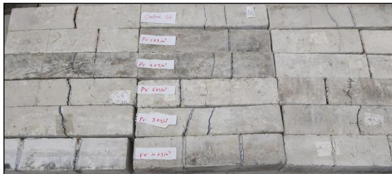
**Fig. 24: The Crack Pattern and Mode of Failure for Prisms with Polyolefin**
