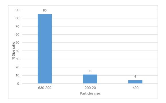
Fig. 3. Distribution of sludge samples' particle sizes.
