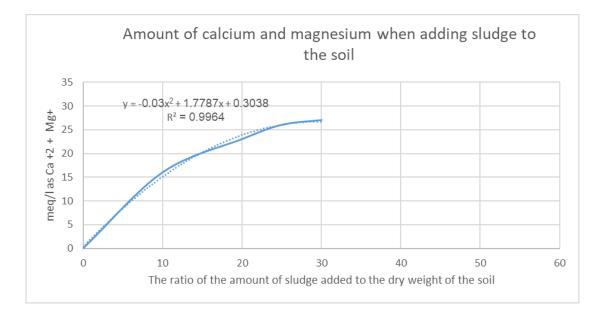
Fig. 6. The relationship between the amounts of sludge added and calcium and magnesium.
