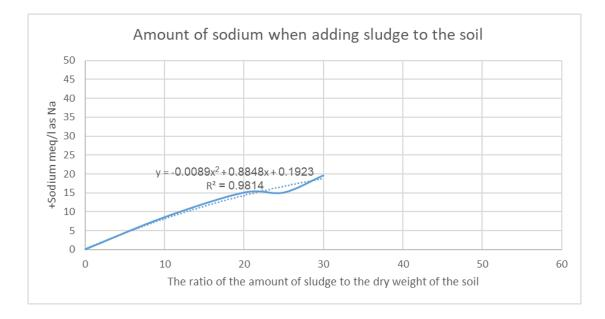
Fig. 4. The relationship between the amounts of sludge added and sodium.
