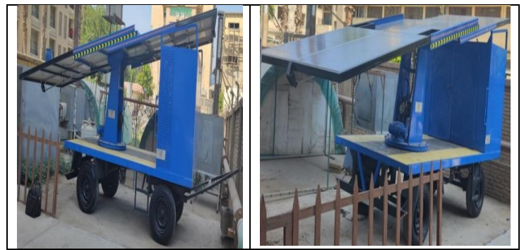
Fig. 16 Final View of the mobile solar water pumping system
