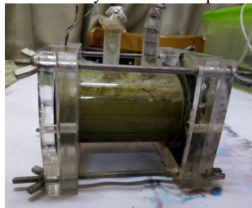
Figure 1: Air cathode single chamber MFC.
