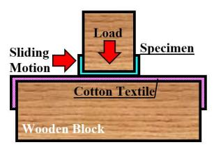
Fig. 2 Arrangement of the teste test procedure.
