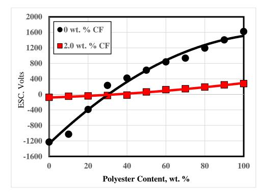
Fig. 5 ESC generated on cotton textile from the contact-separation with PET/PA strings.
