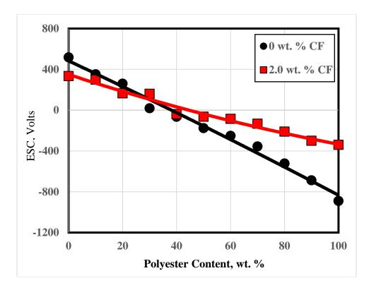
Fig. 4 ESC generated on PET/PA strings from the contact-separation with cotton.
