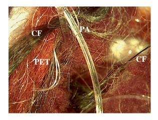
Fig. 3 PET/PA blended by CF test specimen.
