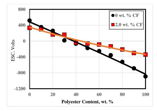
Fig. 7 ESC generated on cotton textile after sliding on PET/PA strings.
