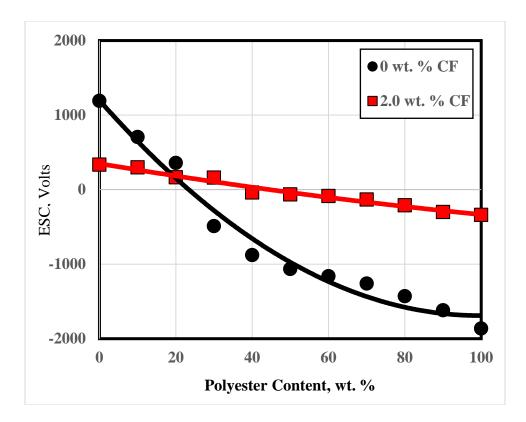
Fig. 6 ESC generated on PET/PA strings from sliding on cotton textile.
