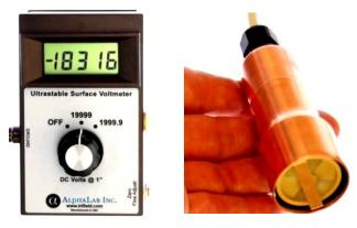
Fig. 1 Electrostatic field measuring device.
