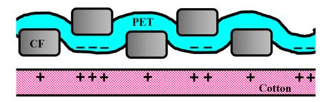
Fig. 6 Representation of ESC generated on the contact surfaces after contactseparation and sliding.
