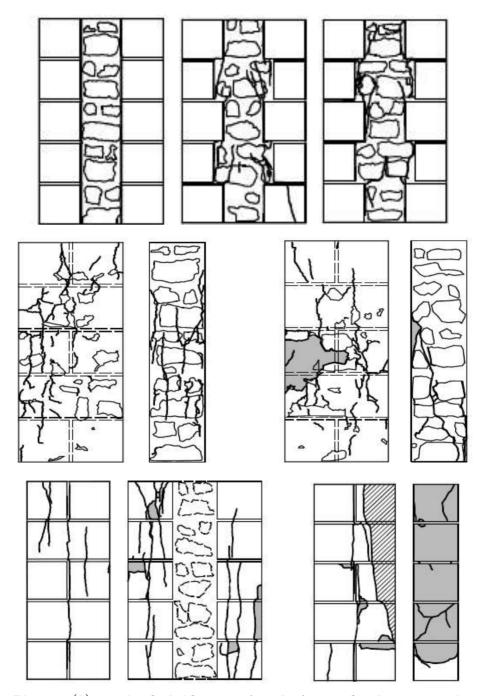
Figure (3) typical failure mode of three-leaf masonry in compression.
