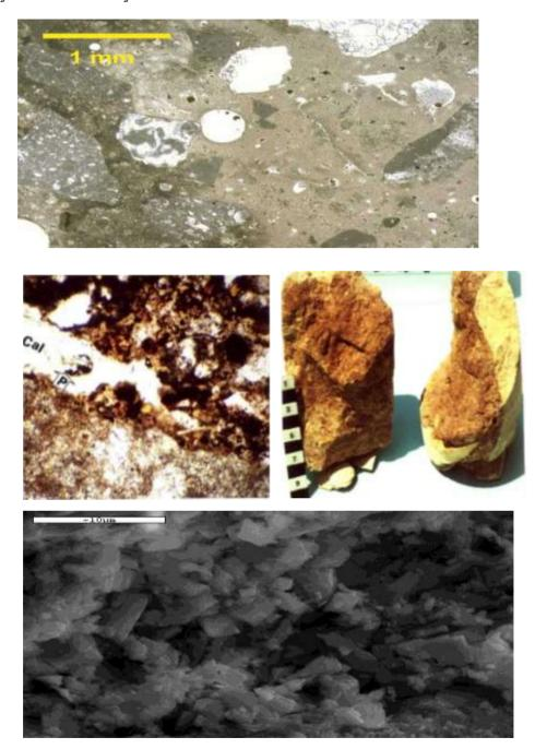
Figure (4) Stereoscopic, polarizing and SEM microstructures examinations of the deteriorated core of rubble infill masonry walls under investigation.
