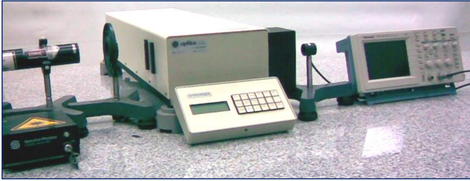
Fig.2. Experimental set-up to measure the spectrum of light sources.
