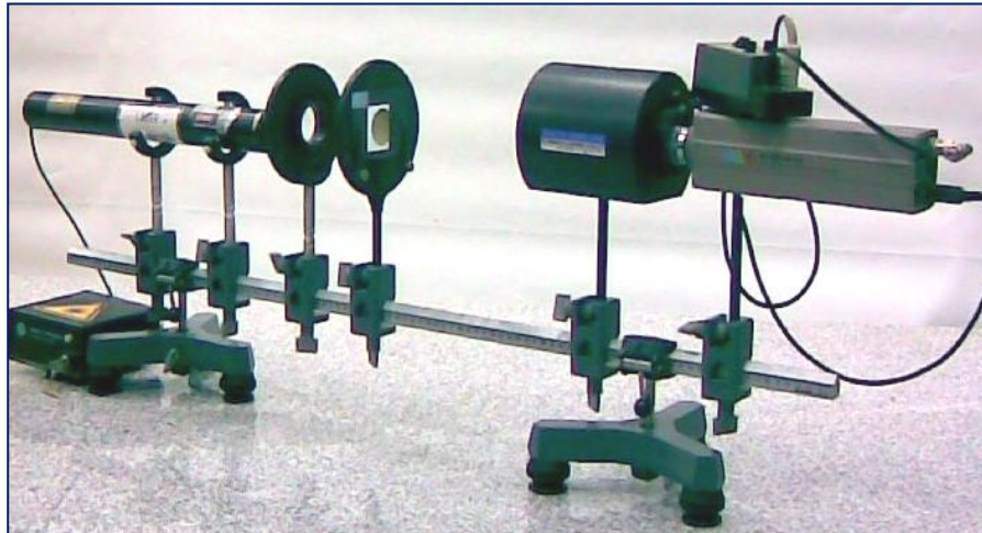
Fig. 5. Experimental set-up for recording speckle pattern
