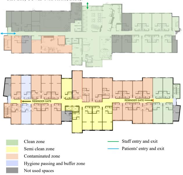
**Figure 4:** Ground and typical floor plan zoning by researcher based on (Performance Work Statement (PWS) Convert a Hotel into a Temporary Alternate Care Site, COVID Non-Acute, 2020).
