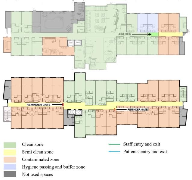
**Figure 5:** Ground and typical floor plan zoning by researcher based on (Performance Work Statement (PWS), Convert a Hotel into a Temporary Alternate Care Site (ACS), COVID Acute, 2020).
