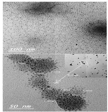
Fig. 1: TEM image of prepared nano chitosan.
