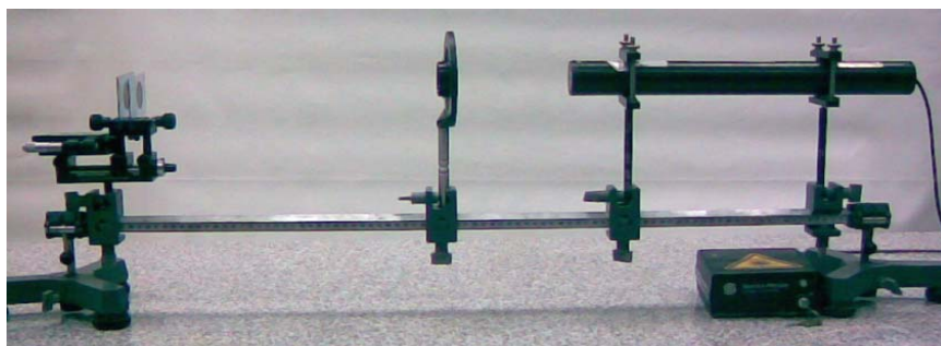
Fig. 4 Experimental set-up for recording Gabor hologram.
