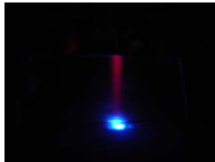
Figure 9. Fluorescence from a chlorophyll-doped elastomer with UV excitation.
