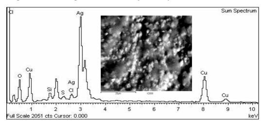
Figure (2) SEM image at magnification2000x of silver and copper alloy shows the metal surface pitted and porous; SEM-EDX pattern shows the alloy consists of 42.02% oxygen, 2.34% silicon, 0.82% sulfur, and 0.54% chlorine, 17.2% copper, and 37.09% silver.
