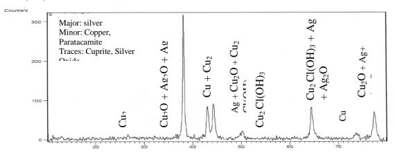
Figure (4) shows the X-ray diffraction pattern of the sample, the corrosion products represented in minerals Silver Ag, Copper Cu, Paratacamite  $Cu_2Cl(OH)_3$ , Cuprite  $Cu_2O$ , and silver oxide Ag<sub>2</sub>O.
