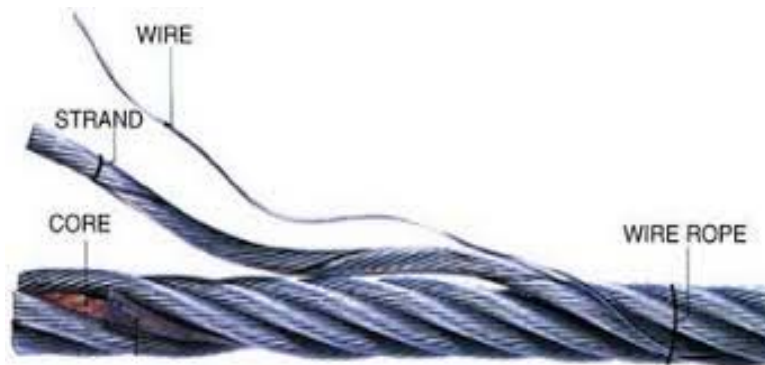
Figure 1. Wire rope construction [6].
