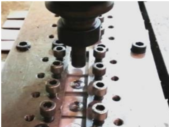
Figure 2. The FSSW process.
