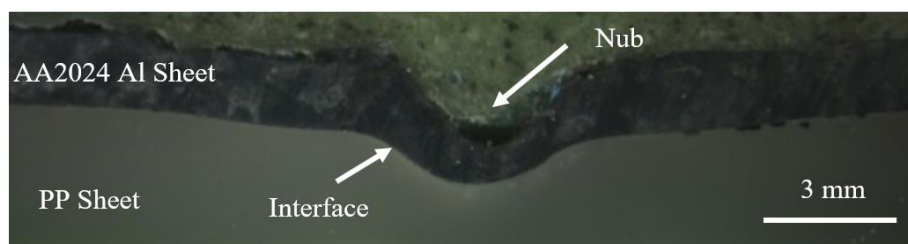
Figure 5. Typical cross-section of FSSW joint illustrating the interface between the AA2024 Al sheet and the polypropylene sheet.
