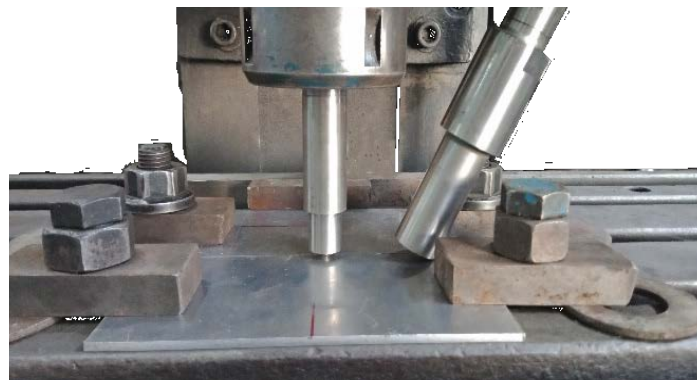
Figure 2. Experimental setups of ultrasonic vibration friction stir welding process.
