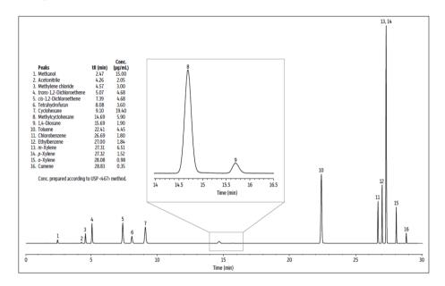
Fig. 5: Typical chromatogram of class 2\_Mix A standard solution.<sup>17</sup>
