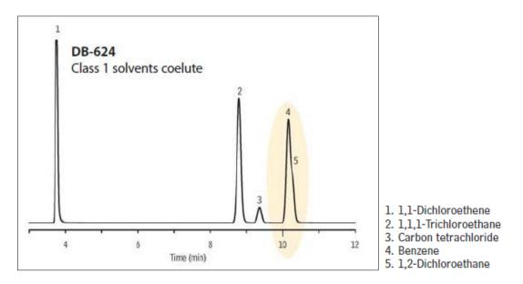
Fig. 3: Typical chromatogram of class 1\_USP standard solution.<sup>16</sup>
