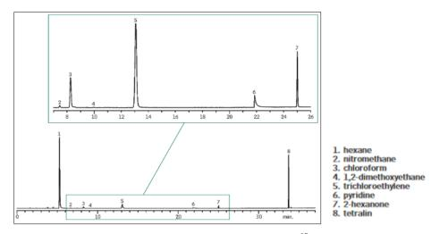
Fig. 7: Typical chromatogram of class 2\_Mix B standard solution.<sup>18</sup>
