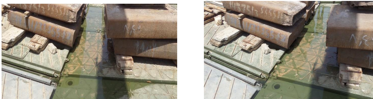
Figure 15: Field draft depth of the bridge system under the second case of static load [1]
