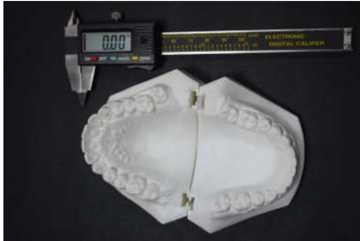
Figure (2): digital caliper for measuring mesiodistal dimensions
