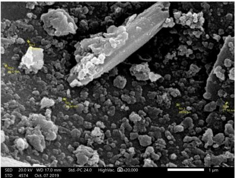
Plate (2). SEM micrograph of Hard biochar
