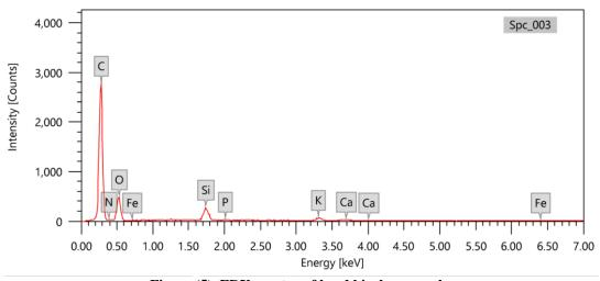
Figure (5). EDX spectra of hard biochar sample
