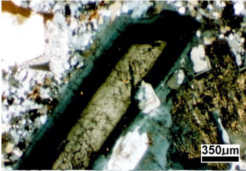
Fig.18:Photomicrograph of andesitic dyke showing zoned crystals of plagioclase phenocrysts forming porphyritic texture
