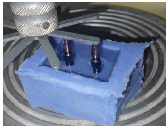
Figure (2): Epoxy resin slowly poured around each implant-abutment assembly.
