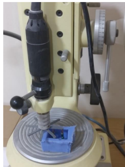
Figure (1): Milling machine surveyor holding two parallel implants during epoxy resin setting.
