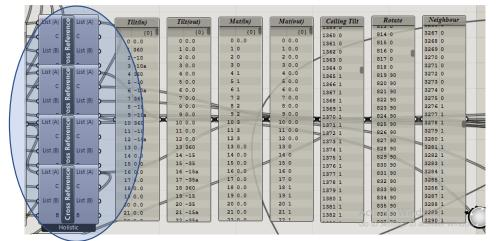
Fig. (4) Modifications parameters for the study modelling which are applied by cross-reference component in Rhino grasshopper.
