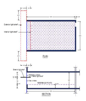
Fig. (1) Hypothetical office building room plan and section is 300 lux (daylight autonomy)
