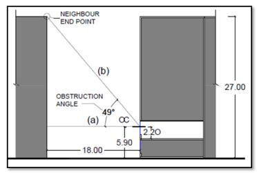
Fig. (2) This figure has define a distance of 18 meter away from the neighbour which make an obstruction angle of  $(49^{\circ})$
