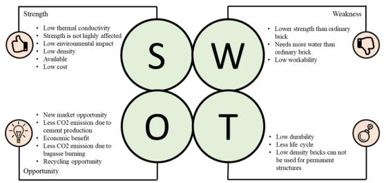
Figure 31. SWOT analysis of brick with bagasse replacement (developed by author, 2019)
