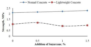
Figure 27. tensile strength of concrete after 28 days (Khalid, 2017)
