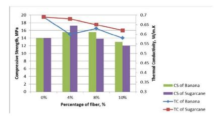
Figure 30. Compressive strength and thermal conductivity relationship of sugarcane bagasse and banana trunk fiber (Aminudin, 2017)
