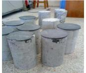
Figure 18. Concrete blocks after curing (Kumari, 2015)
