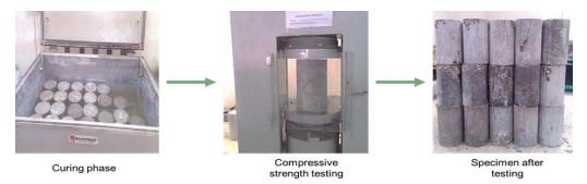
Figure 22. steps of concrete specimen from curing to testing and its final shape (Mangi, 2017)
