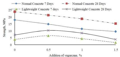
Figure 26. Compressive strength of concrete with sugarcane bagasse (Khalid, 2017)
