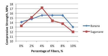
Figure 29. Compressive strength against percentage in comparison with banana trunk fiber and sugarcane bagasse (Aminudin, 2017)
