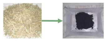
Figure 17. Combustion treatment process (Kumari, 2015)
