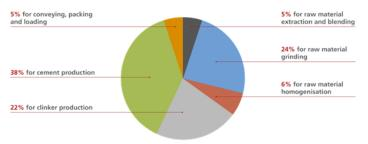
Figure 15. Energy demand of the cement production process (cembureau, 2018)
