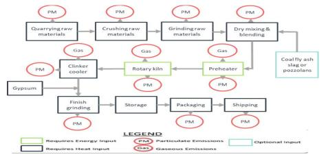
Figure 3. Cement production process and emissions, (Eštoková, 2012)
