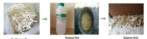
Figure 25. Sodium Hydroxide NaOFTW8934Ster treatment method steps (KHaftdh29917)
