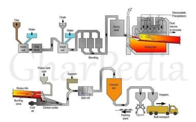
Figure 14. cement manufacturing process (gharpedia, 2018)
