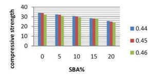
Figure 19. Compressive strength of different SBA percentages and different W-C ratio (Kumari, 2015)
