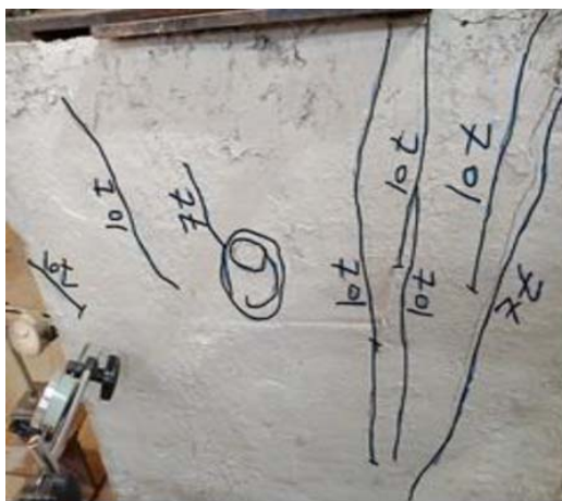
Fig. 15 Cracking patterns of all the tested light weight panels under compressive.
