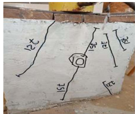
Fig. 15 Cracking patterns of all the tested light weight panels under compressive.
