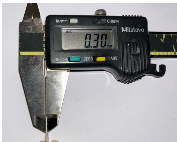
Figure 1: Digital Micrometer is used for checking veneer's marginal thickness of 0.3mm.
