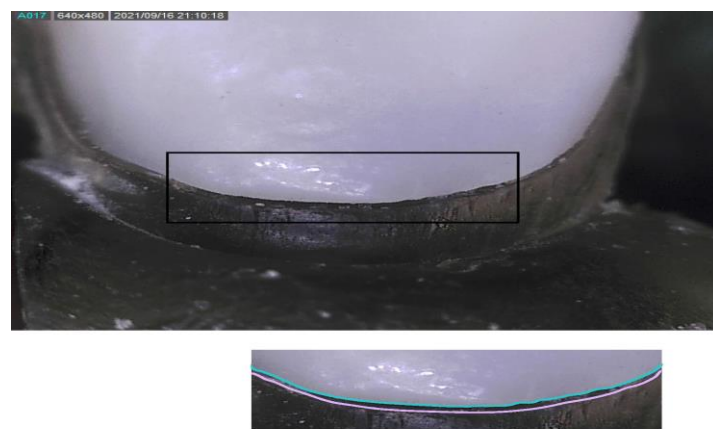
Figure 3: The gingival margin under stereomicroscope of IPS e.max veneer made of 0.3mm marginal thickness produced by MCXL milling machine.
