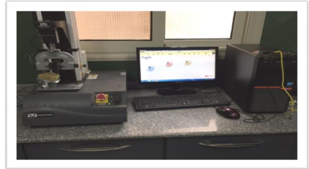
Figure. Specimen fixed to the customized lower compartment of computer-controlled universal testing machine.
