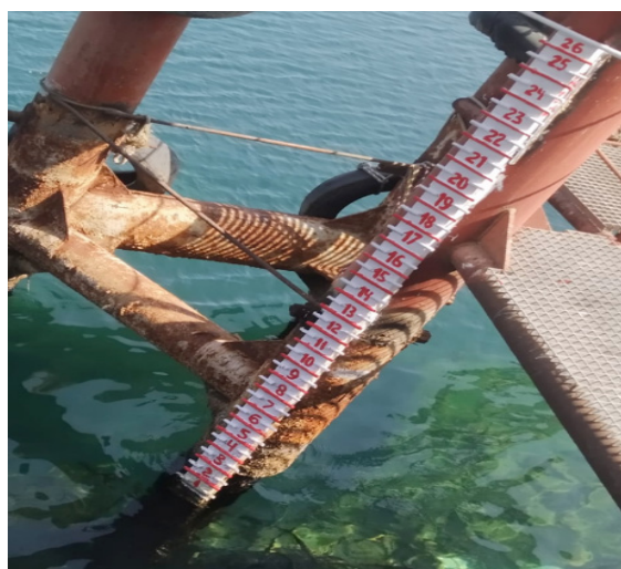
Fig. 1. Tamasa is used to measure the water level at the Sea Hydrometeorological Station of the “Neft dashlari” in the Caspian Sea.
