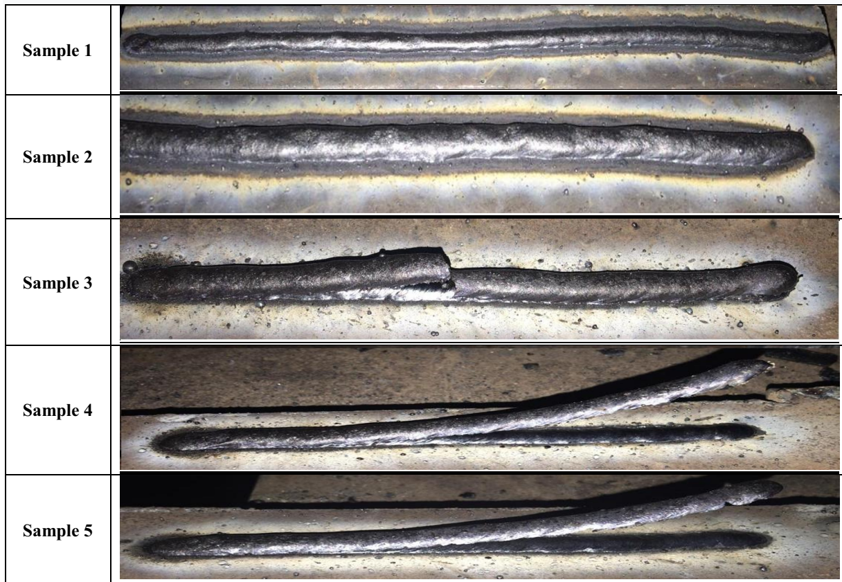
Figure 2. Slag and welding profile
