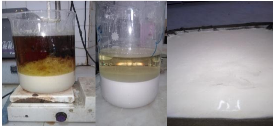
Figure 1. Thorium oxalate precipitation after oxalic acid addition.
