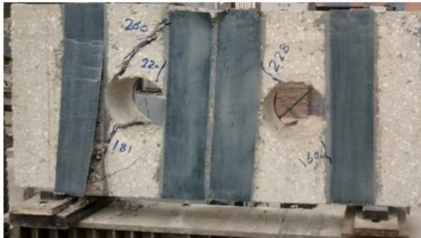
B8-CO-F: Diagonal-shear splitting failure
