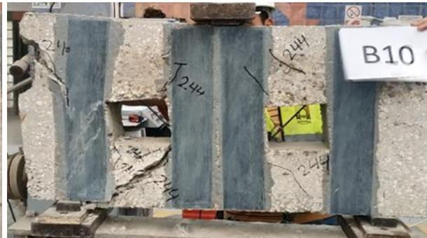
B10-SO-F: Diagonal-shear, concrete
