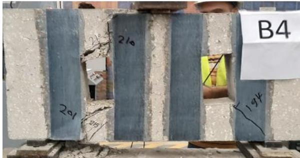
B4- RO-V-F :Diagonal-shear splitting failure
