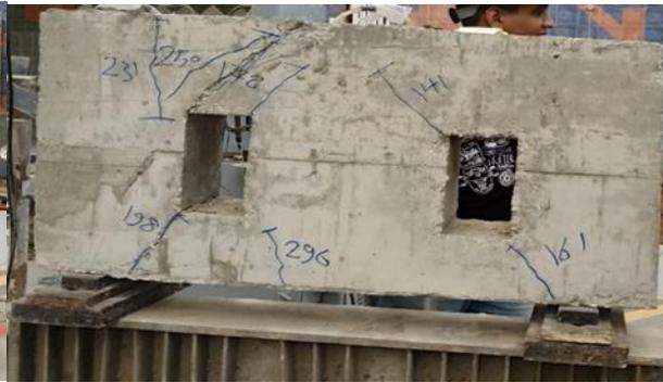
B3-RO-V: Diagonal-shear splitting
