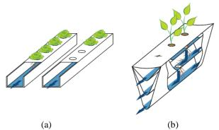
Figure 7. (a) Illustration of traditional NFT system and (b) a multilayer NFT trough, developed and marketed by New Growing Systems (NGS), Spain (Maucieri, Nicoletto et al. 2019)
