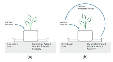
Figure 5. Scheme of an open cycle (a) and closed loop systems (b) the source (Maucieri, Nicoletto et al. 2019)
