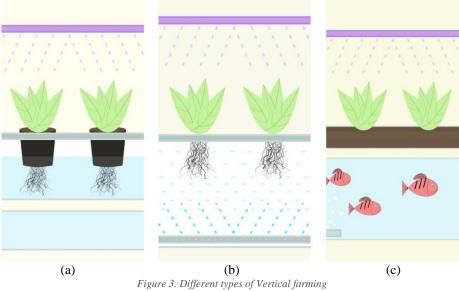
Figure 3. Different types of Vertical farming (a) hydroponics – (b) aeroponics– (c) aquaponics Source: (Denisa 2022)
