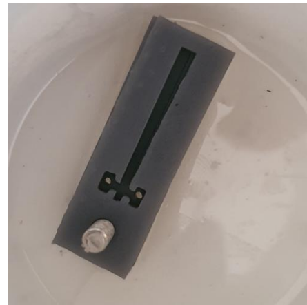
Fig. 6 mold with silicone poured into
