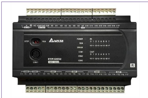
Fig. 6 Programmable Logic Controller (PLC)
