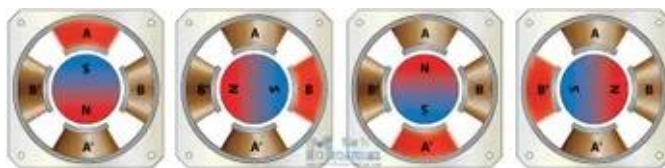
Fig. 5 Stepper Motor Operating Principles
